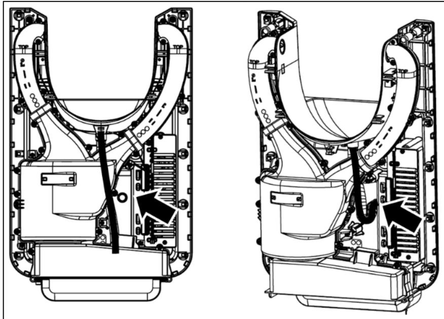
Fit the hose supplied with the machine to the water drain at the rear of the machine. Mount the machine on the wall keeping in mind that the hose mounted on the machine must enter the drain in the wall.
