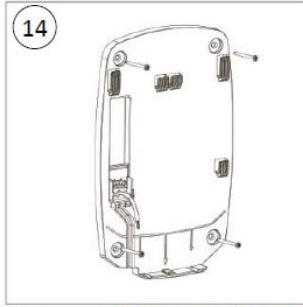
14 Screw the Plug-in base to the wall(x4)
